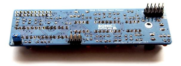
The blue jumper selects the speed range of the module. With the jumper in place the module runs slow, barely touching audio range, but with modulation cycles down to 10-15 minutes. With the jumper removed it runs up to audio range, but the low end is reduced.
