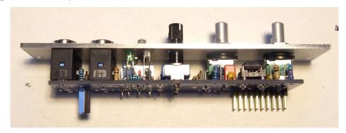
Cut off the pins of the jacks as flat as possible, otherwise they may touch the caps on the lower PCB later on. Be careful, the legs of the jacks are like small powered high energy projectiles when cut off with wire cutters! (You'll shoot your eye out!) Ignore the missing bolt on the following pictures.
